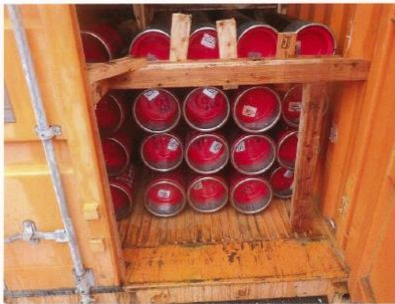
Final stowage and securing condition at door end
