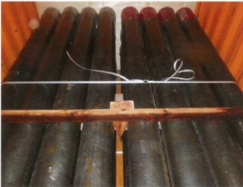
Final stowage and securing condition at front end
